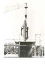
Headfirst into the treatment bath: Dürr presents the VERTAK process. This involves car bodies being immersed vertically into a silo-shaped tank to receive their protective coating against corrosion.
